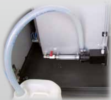
Built-in tank draining pump for used cooling medium. To be disposed of as cooling emulsion.
